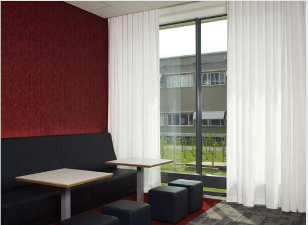
The fullness and wave depth of the curtain depends on the selected glider cord and the applied spacing between the curtain hooks. The stack depth varies between 8cm and 14cm.
