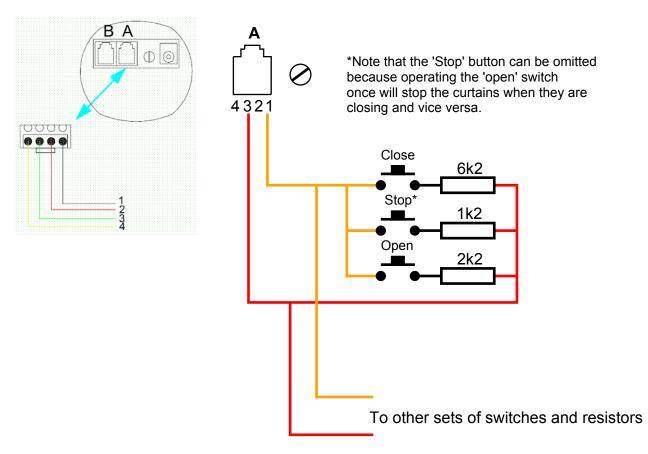
Several sets of buttons and resistors can be used, but if two buttons are pressed at the same time, incorrect operation might result.
